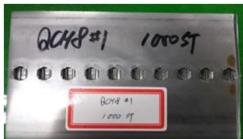
Fig. 3 Pocket shape blank for VCT Inner plate parts
