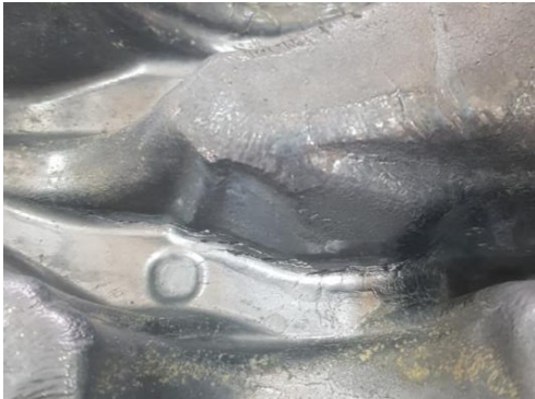
Fig. 2 Crack occurring in a die corner
