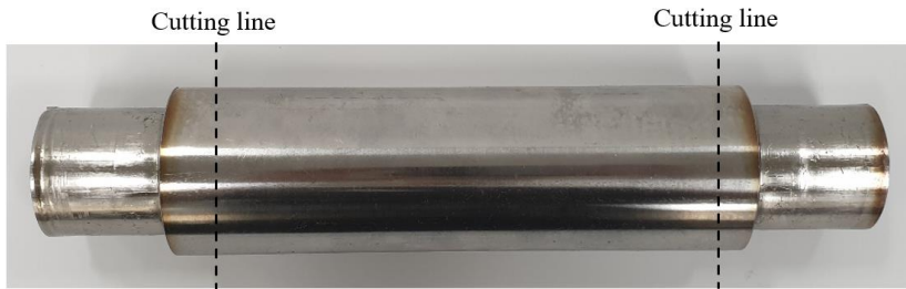
Fig. 2. Final shape after hydroforming
