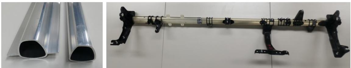
Fig.1 Porthole extrusion products and assembled cowl cross member
