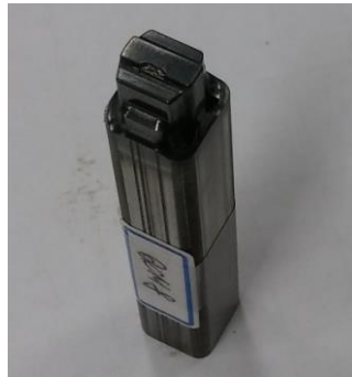
Fig. 2 Pocket punch for VCT Inner plate parts
