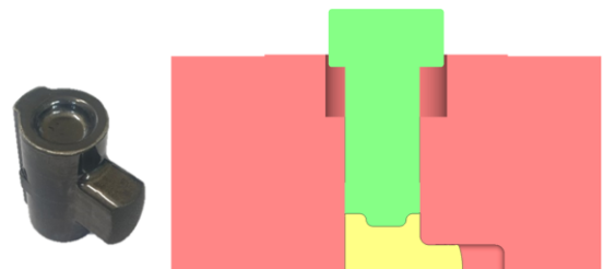
Fig. 1 Ball Nut and 1/4 model for FE-simulation
