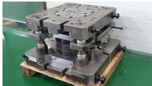
Fig. 1 Outer plate die for fine blanking
